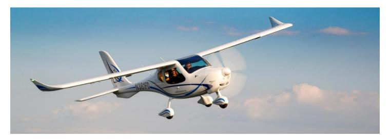
The F2 was designed specifically for international CS-23/Part-23 certification and to meet the ASTM F3180 low-speed flight characteristics of fixed-wing aircraft standard for slow flight characteristics, spinning, and stall warning. The sculpted winglets reduce drag, improve climb, stability and cruising range. The smooth cantilever strutless wing also reduces drag and allows maximum visibility from the cockpit.
